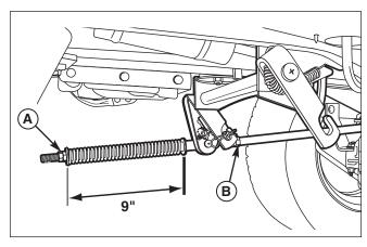
Figure 23. Lift Rod Spring Adjustment A. Front Lift Rod Nut
